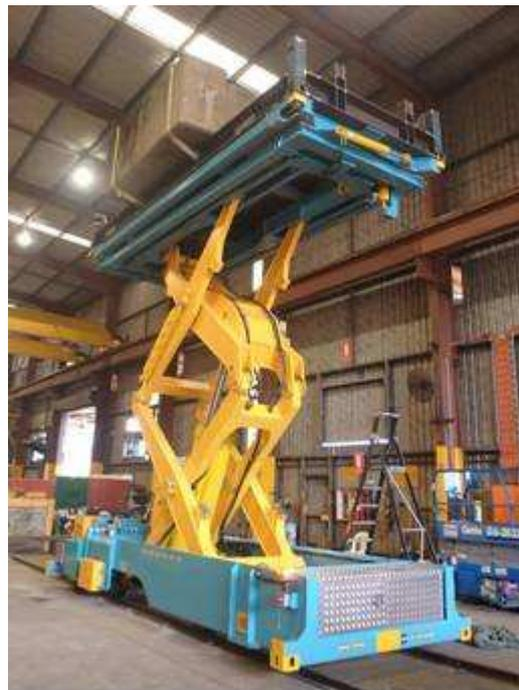
**Schenck Process ProLift undergoing stability testing**
