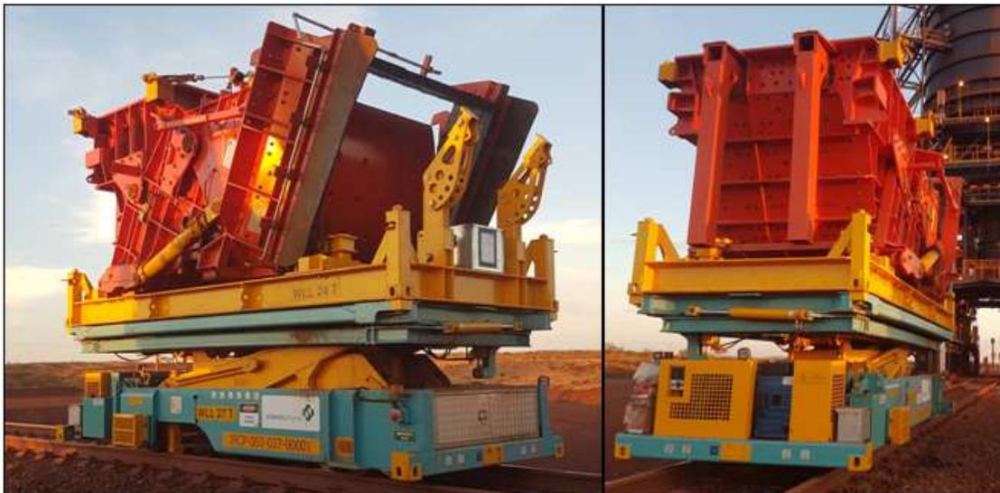
**Schenck Process ProLift approaching a train load out with a new chute**
