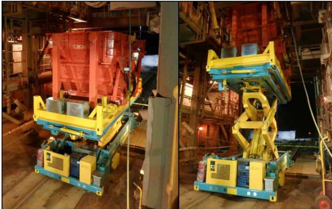
**Schenck Process ProLift in the train load out lifting chute into position**
